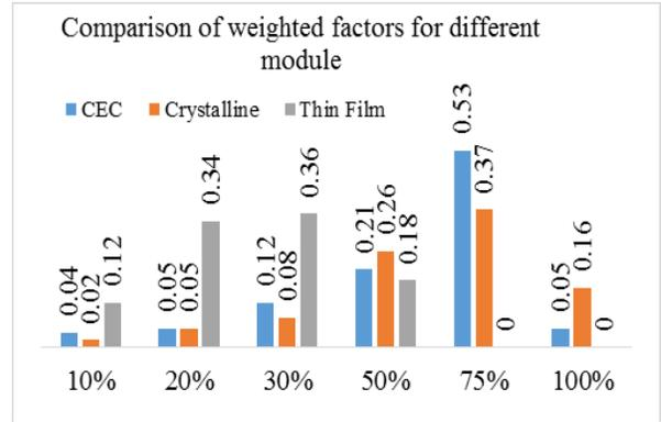
Figure 6. Weighted coefficients for two different modules for same location i.e. Hainan,China.
