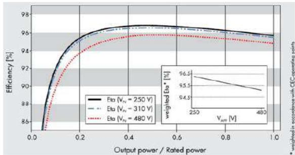
Figure 1. Efficiency plot of commercial PV inverter [1].
