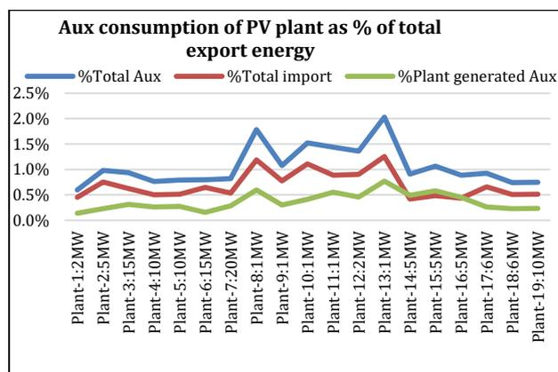
Fig 1. Aux consumption of plant in broad view ranging from 1MW to 20MW
