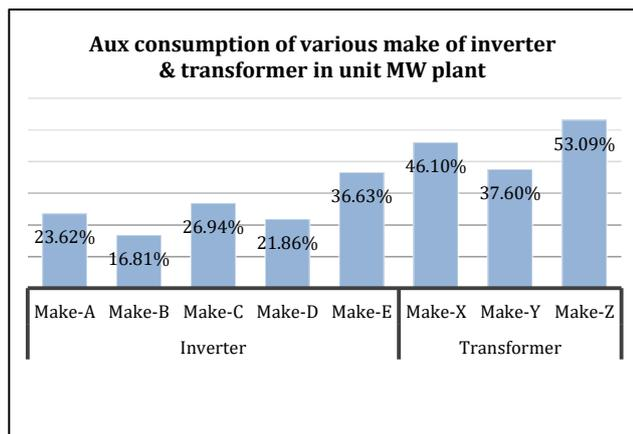
Fig 3. Aux consumption of Inverter & No load loss in transformers
