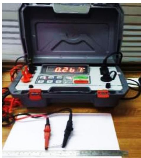
Fig.1 Measurement setup for micro-ohmmeter
